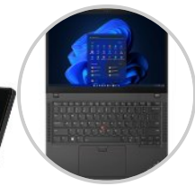
TrackPoint pointing device and glass-like Mylar® surface multi-touch touchpad, 61 x 115 mm (2.40 x 4.53 inches)
