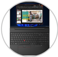
TrackPoint pointing device and Mylar surface multi-touch touchpad, 68 x 115 mm (2.68 x 4.53 inches)
