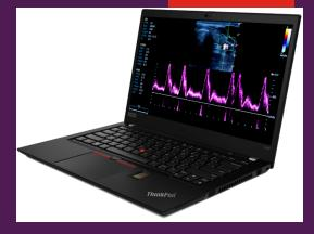
User authentication technologies include a US federal-approved FIPS-201 fingerprint reader, an integrated RFID/NFC reader so users can login with an employee badge, and an optional infra-red camera.
